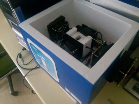
Fig. 2. Photograph of the polystyrene thermal box and spectrometer.
